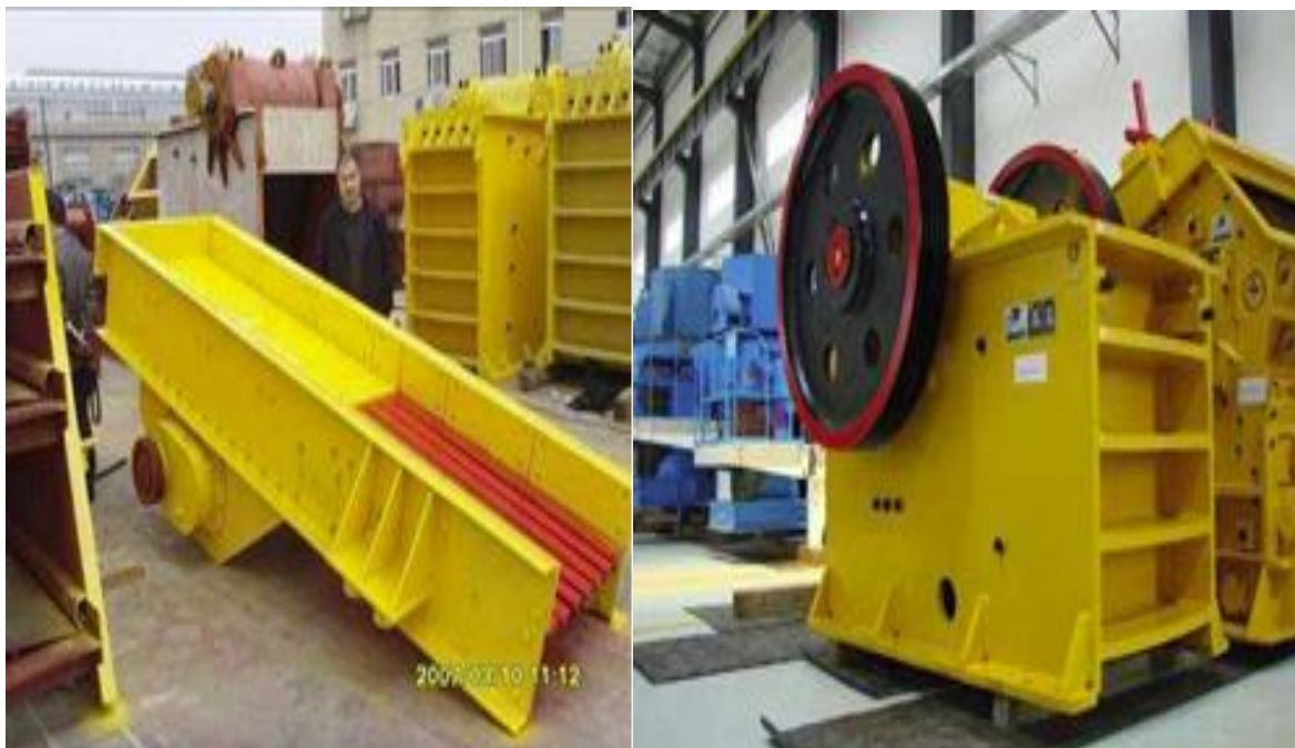
Figure 4-4 Vibratory Feeder & Jaw Crusher
