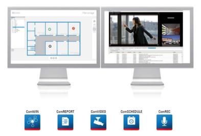
control desk station. PA announcement zones can be selected from GUI map and pre-recorded message can be played in that selected area or manual announcement can be broadcasted in selected area through hardware control desk station microphone. Further there is submodules as following to support efficient handling of PA System,
